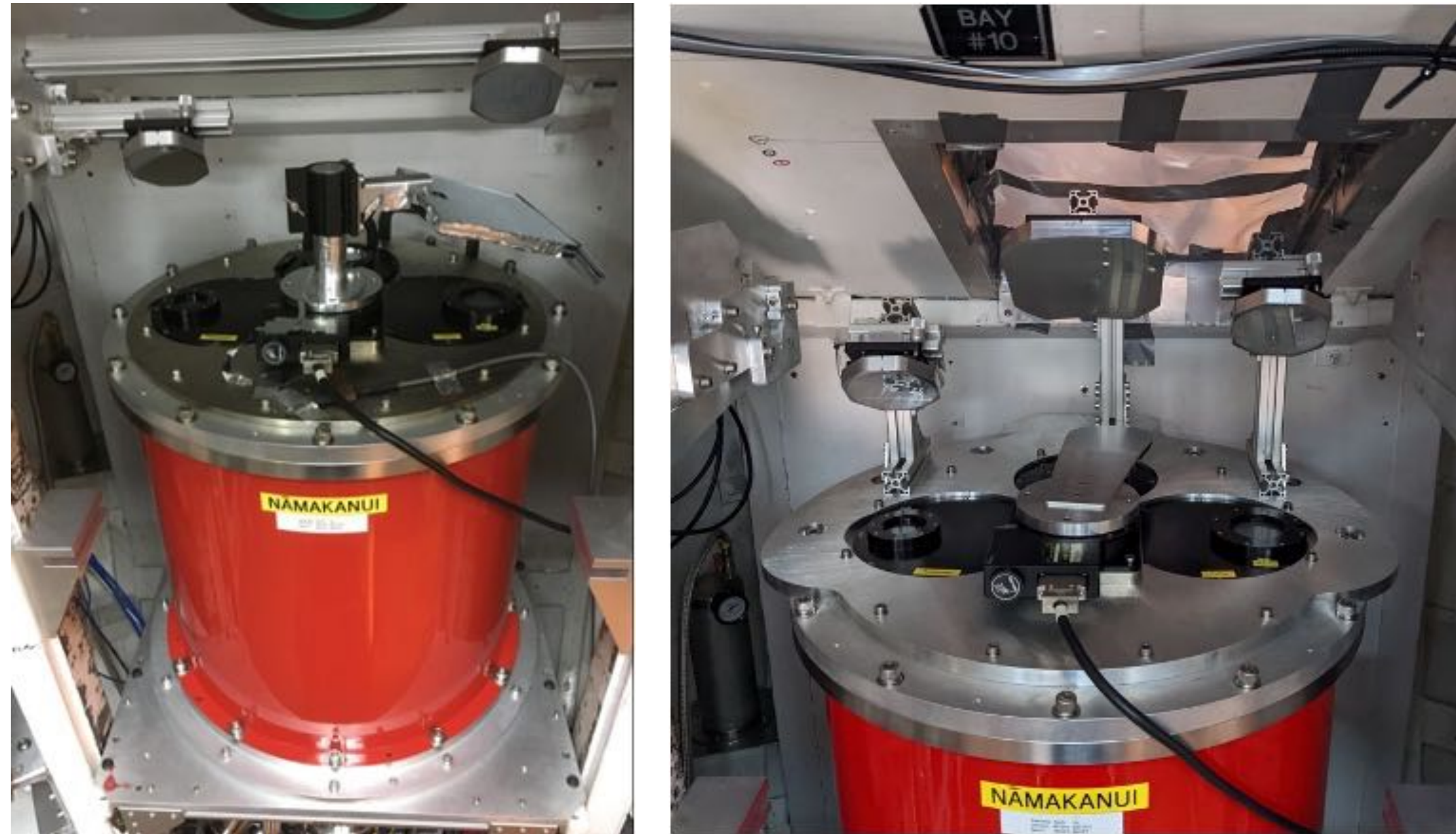
Figure 1. View of Nāmakanui instrument installed in cabin. Left picture shows the initial coupling mirror and ambient load mount, and right picture shows current mount. Three receiver inserts located in the Dewar at left forward (ʻĀweoweo/345GHz receiver), center behind (ʻAla`ihi/86GHz receiver) and right forward (ʻŪ ū/230GHz receiver). Each relay/coupling mirror is mounted above each receiver window. Rotation stage supporting the ambient load, is located at center on top of the Dewar.
